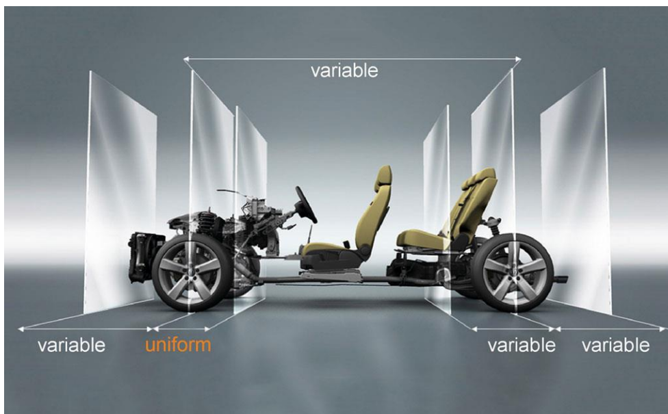
Figure 2.10. Volkswagen's new MQB platform (Colwell, 2012)
